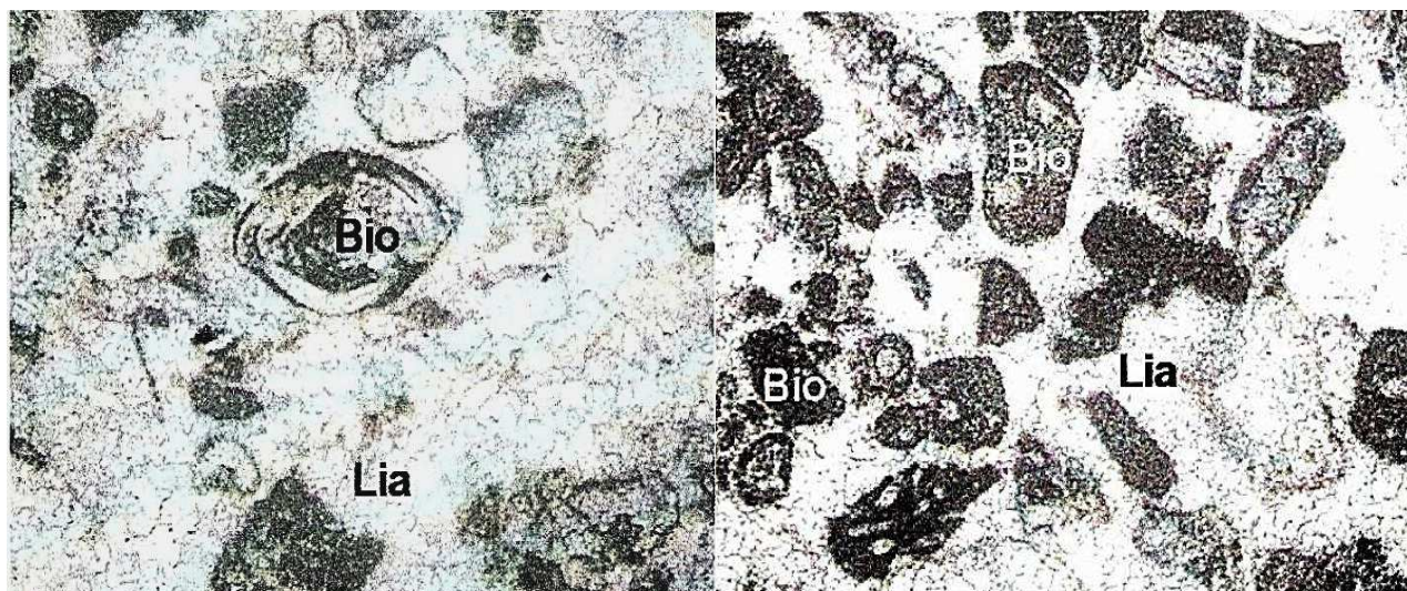
Figure 5. Organogenic limestone (x 257; N II; x = magnification of image; N II = normal light image)
